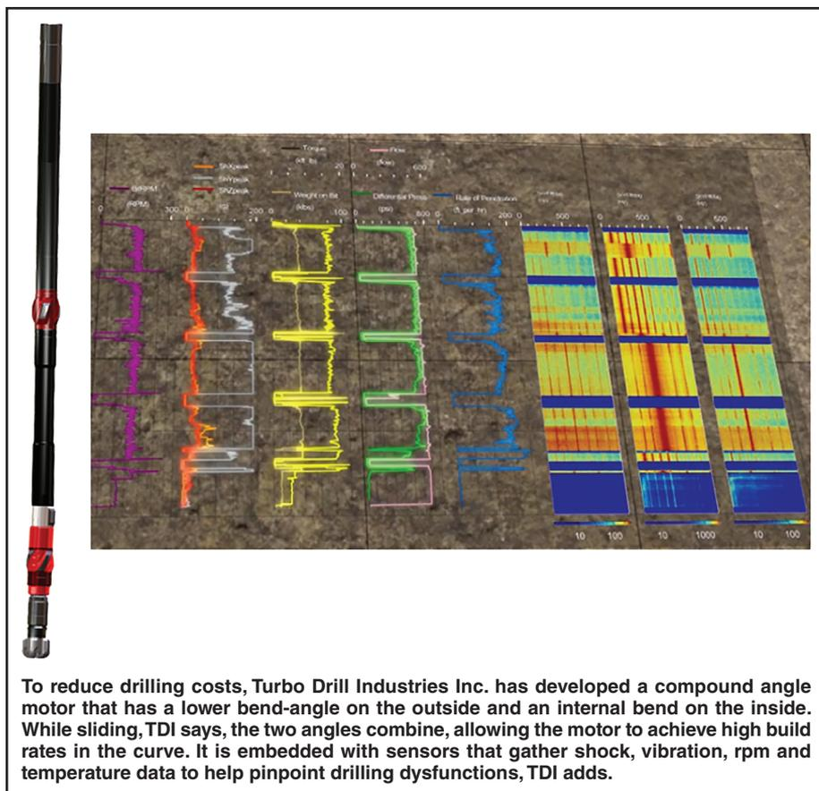
To reduce drilling costs, Turbo Drill Industries Inc. has developed a compound angle motor that has a lower bend-angle on the outside and an internal bend on the inside. While sliding, TDI says, the two angles combine, allowing the motor to achieve high build rates in the curve. It is embedded with sensors that gather shock, vibration, rpm and temperature data to help pinpoint drilling dysfunctions, TDI adds.
